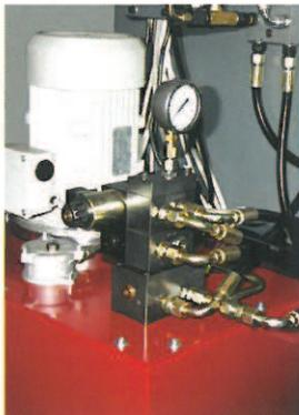
Separate hydraulic system with control column. 4/2 and 4/3-way directional control valves 24 V DC according to European Standard.
