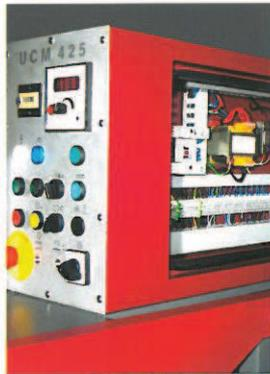
Electric control according to VDE with electric cutting pressure monitoring and piece counter.
